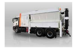
RSP suction superstructure on a 3-axle-chassis. Its compact design and performance capabilities allow the ESE 6 to be used everywhere. The collection tank holds either 6 m³ or 8 m³. Single or twin fans and all types of suction hose carriers can be installed.
