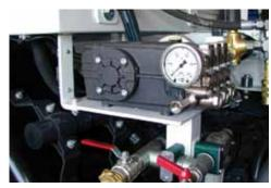
ESE 6 High-pressure water system inclusive of stainless steel hose reel
