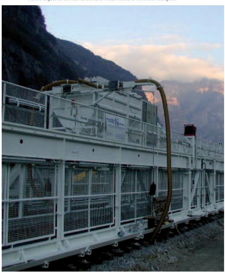
For cleaning work in the world-famous city of Venice, RSP developed a suction system by the name of Leonardo. It was put to work clearing Venice's clogged canals of sediment and waste. When developing the system, particular focus was placed on a low-noise design which would benefit residents and tourists alike.
